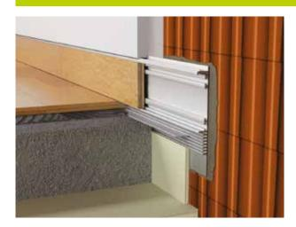
BFZ is a construction profile that allows you to create a flush-to-the-wall baseboard with the same material as the flooring. In the lower part there are special grooves, designed to allow the insertion of a linear profile which will help to determine the level of the screed and ensure perfect positioning of the heights of doors and windows.
